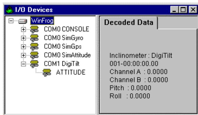
The Decoded Data section of the I/O Devices window displays the raw data being received from the DataMate. These are listed under Channel A: ( $2 \cdot \sin\theta$  value-pitch); and under Channel B: ( $2 \cdot \sin\theta$  value-roll).
